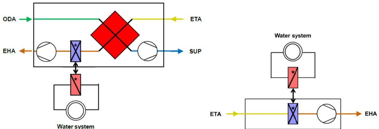
**Concerning RVUs**, it is considered that BVUs equipped with a heat pump for heat recovery only (same as 'heat transfer being additional to heat recovery') do **not** fall under Regulation 1253/2014. Figure 2 show an example of such product
